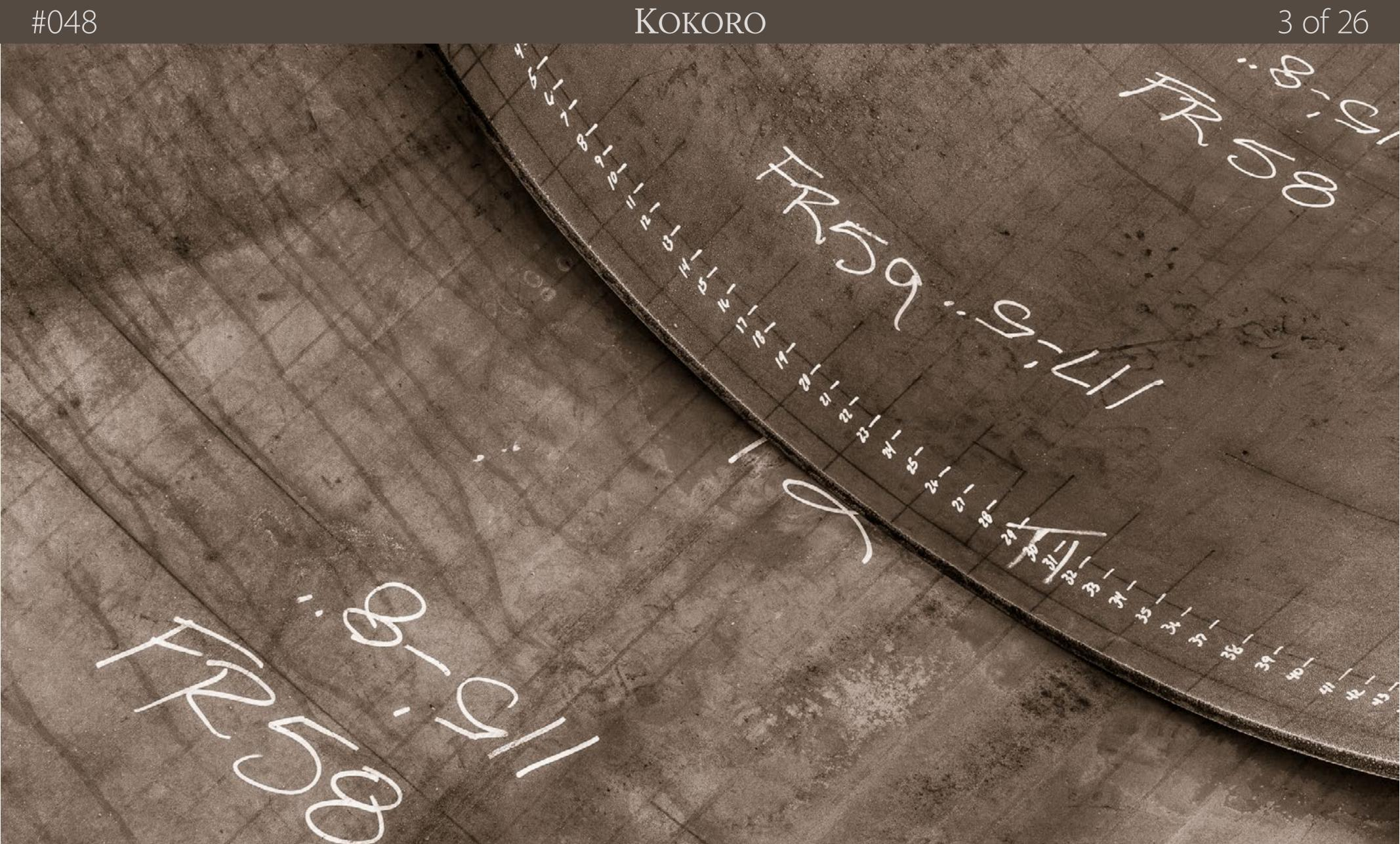
It starts with piles of cut steel, shaped to a tolerance of 1/32", each weighing more than a man can handle, no two of them exactly alike.
